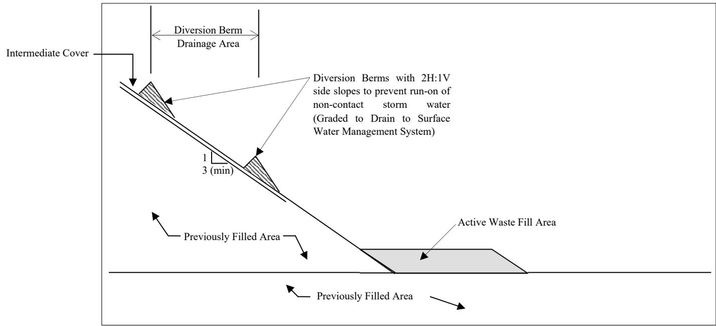
**Figure 1. Typical/Schematic (Conceptual) of Phased Active Fill Area Section (portraying possible conditions where diversion berms may be used) (Not to Scale (NTS))**
