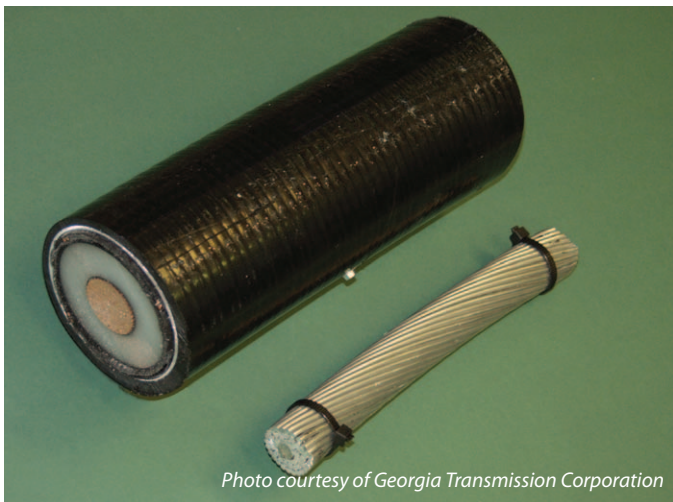
Underground cable and smaller overhead conductor
