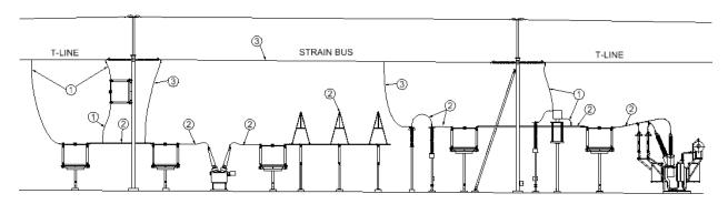
① T-LINE TO SUBSTATION EQUIPMENT - RATE ONLY FLEXIBLE CONDUCTORS PER TRANSMISSION LINE RATING METHODOLOGY SECTION; DERATE CONDUCTORS WHEN CONNECTED DIRECTLY TO:
